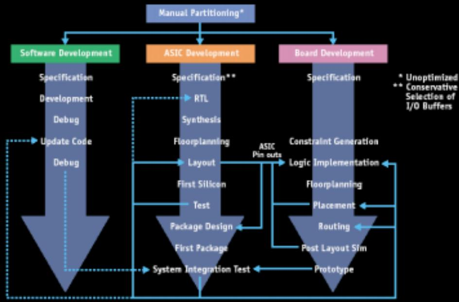
Traditional IC, package and board design are separate processes with many iterations built into each. The results are sub-optimal IC pin outs, longer board design cycles, and board designs that eat into the performance that the IC design team worked so hard to achieve.
