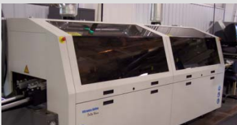
Vitronics Soltec Delta lead-free wave solder with computer control allows us to store and quickly set up the best process for each board.
