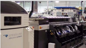
Philips Assembléon high-speed SMT line places 60,000 parts per hour; handles parts as small as 01005.
